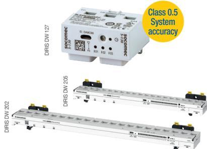
**DIRIS Digiware S** is a multi-circuit current measurement module with 3 integrated sensors and allows the monitoring of three-phase or single-phase circuits up to 63 A.
